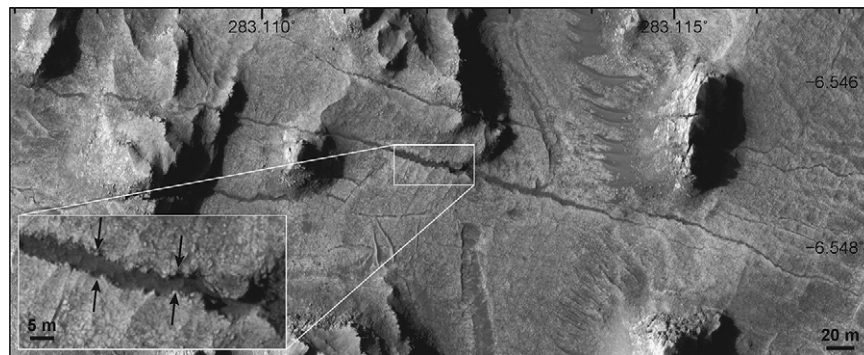
Fig. 17. Joints within the layered sedimentary deposits in west Candor Chasma, Mars. Maximum opening displacement is exhibited near the mid point of each joint. Inset shows examples of asperities along the joint walls that are used to measure the distribution of displacement. HiRISE image PSP_001918_1735, with illumination from the upper left. Inset is at full image resolution (26 cm/pixel).
